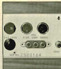
DIN-contacts for radio recording and playback through radio or for remote loudspeakers. An output for Free Head.
