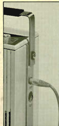
Tandberg Portable Radio Series 3-1 and 3-3 can be connected to the AC-mains by means of a Tandberg Battery Eliminator, which is plugged to the AC-mains and connected to the radio by means of a lead.
