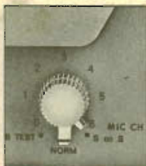
A double control knob for playback on both channels. Sound-on-sound selector with 3 positions.
