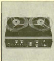
The tape recorder can be used with 7'' spools when cover is removed. 5'' spools with cover in position.
