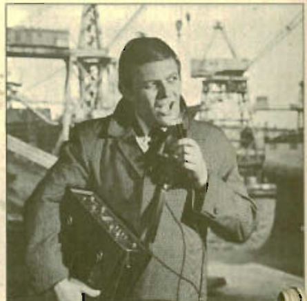
The recorder can be carried and used in a sturdy practical shoulder bag. Pocket for tape and window for spools.
