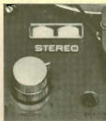
Electronic beam indicator ("magic eye" with slow backward movement ensures correct recording level.
